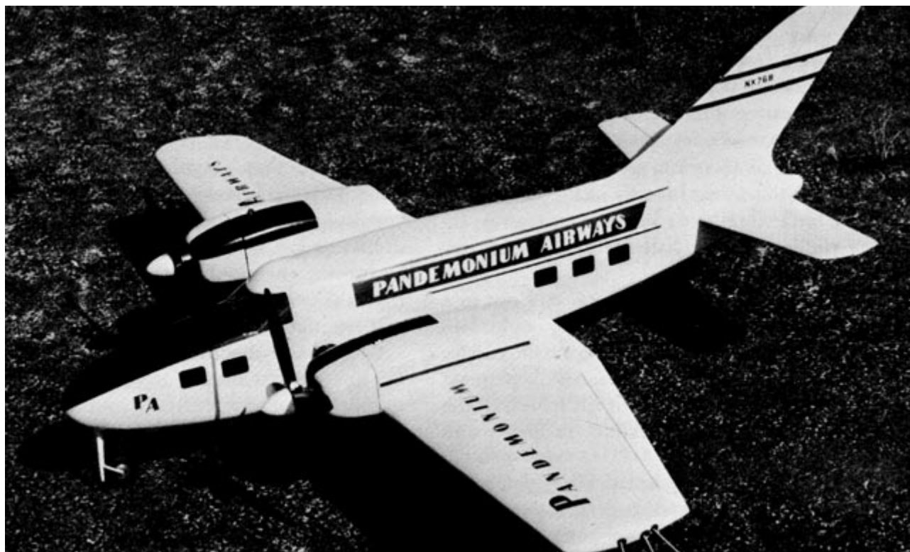
A twin-engined C/L job with clockwork retracting gear
