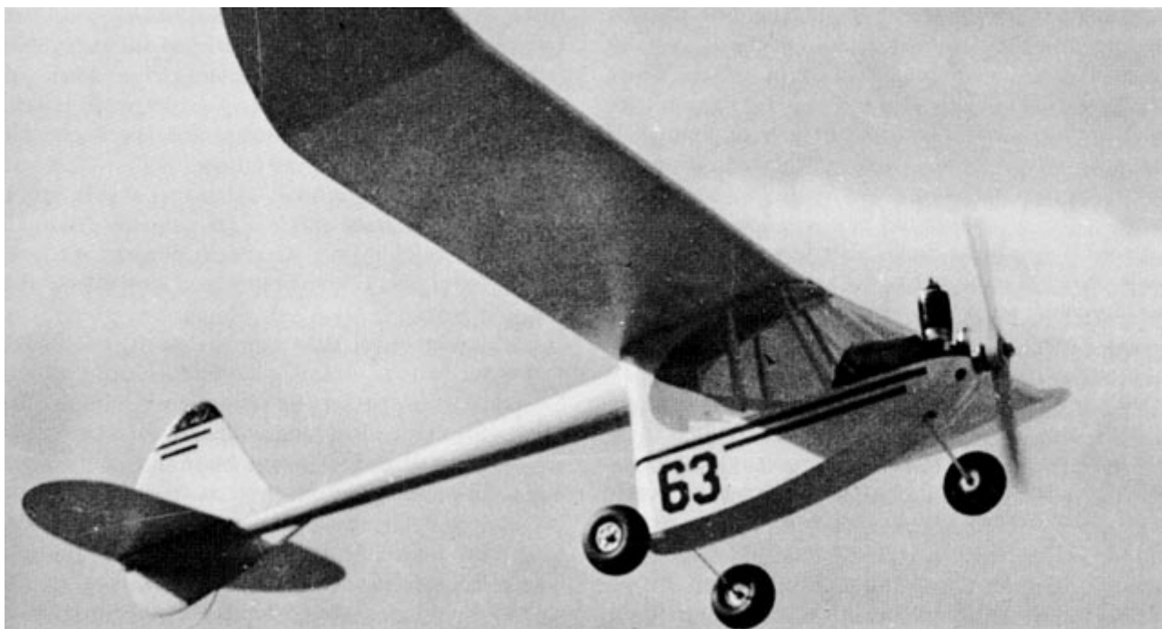
Figure 3.1: A pod-and-boom job with tricycle landing gear. A pod-and-boom job with tricycle landing gear.
